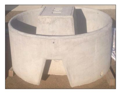
The round troughs can be installed with an optional concrete float protector which stands in the base of the trough and has a cut out that sits over the inlet recess ledge. The weight is approx. 250 kg and saves the float valve from damage if stock get into the trough
